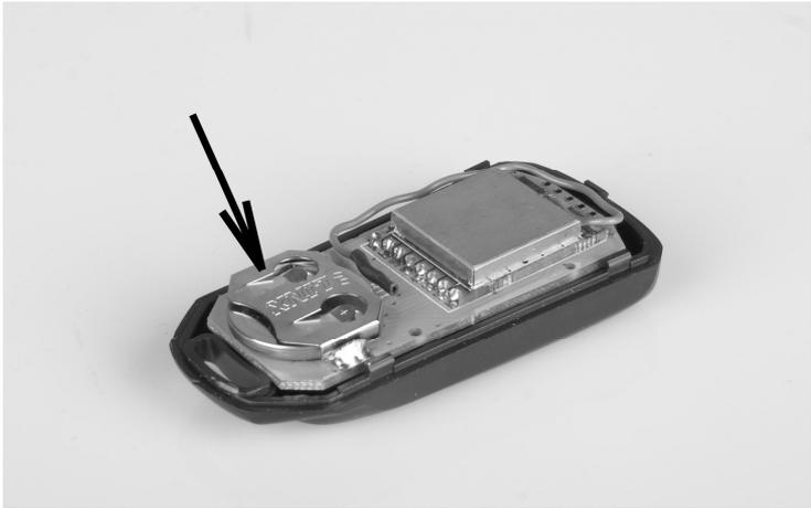
4. Locate the battery and carefully remove it from the board by sliding it out of the holder. Note battery orientation as you remove it as the new battery must go back in the same way (positive (+) side is up, negative (-) is down).
